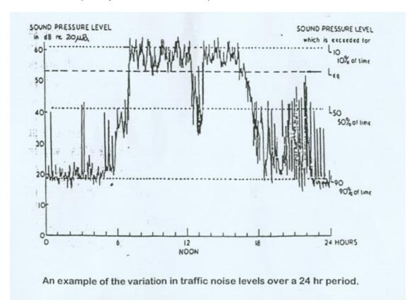
• L<sub>A10,T</sub>: The A weighted level of noise exceeded for 10% of the specified measurement period (T). It gives an indication of the upper levels of fluctuating noise such as that from road traffic. L<sub>A10.18h</sub> is the arithmetic average of the 18 hourly L<sub>A10.1h</sub> values from 06.00 to 24.00.
