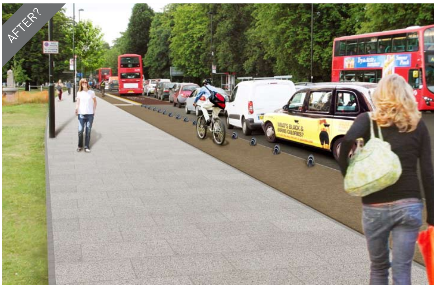
The Mall, looking west from near the North Circular towards Ealing Town Centre: reusing existing, unnecessary and inefficiently used carriageway to create a protected cycle track to link with the existing separated track just beyond the bus stop. The bus stop itself is lightly used. The existing eastbound protected cycle track (on the north side of The Mall) will also be improved.
