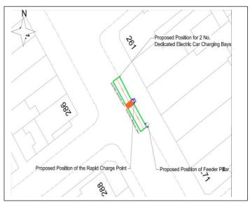
The charge point can deliver a supply of up to 50kWh AC and can function 24 hours a day.
