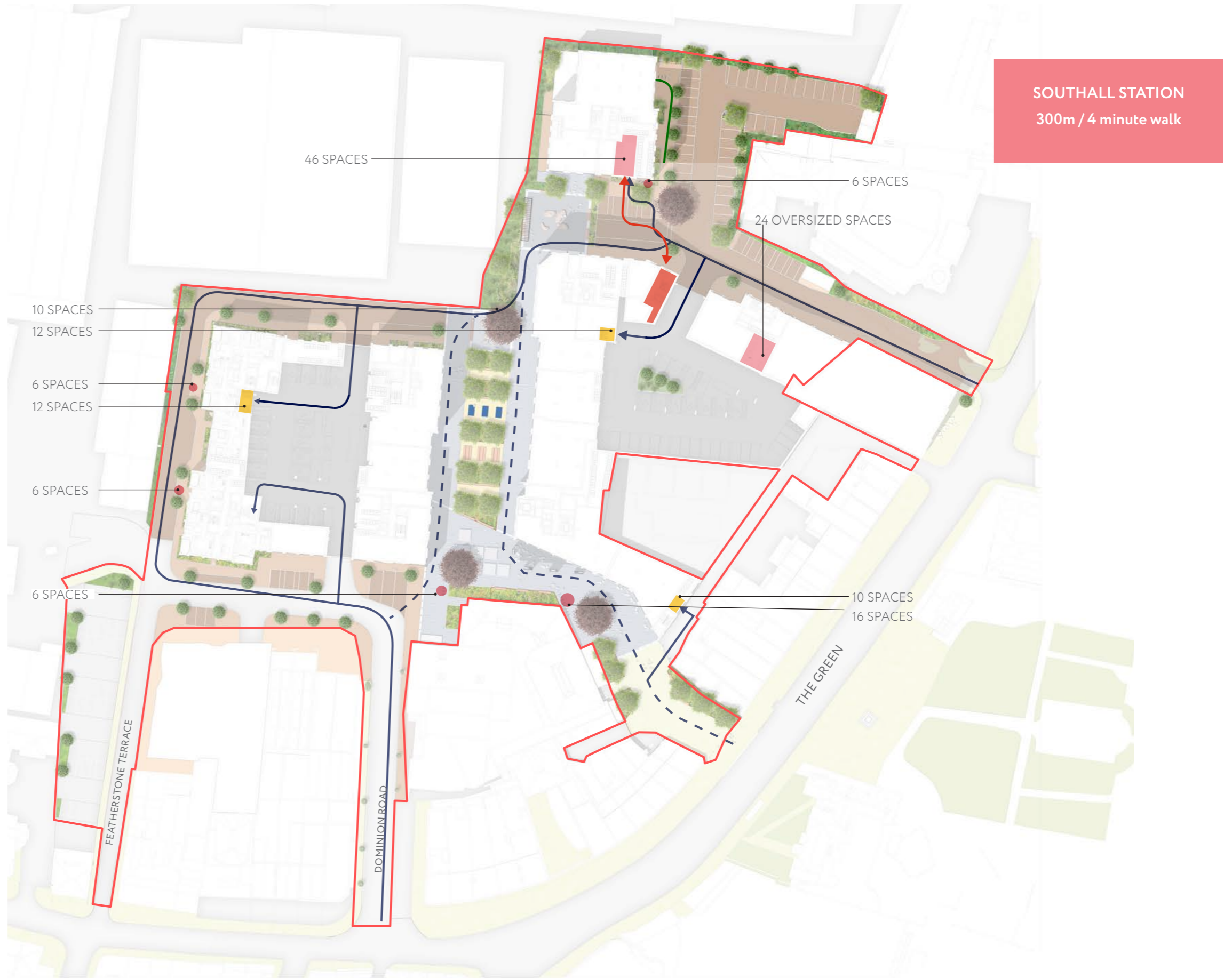
FIG. 6.3 - GROUND FLOOR LEVEL CYCLE STORE (84 SPACES)
