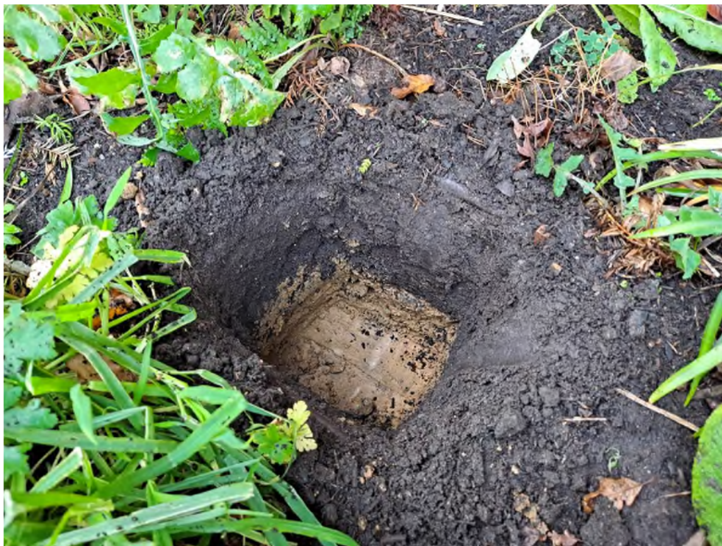
Plate 6: North side – trial hole 0.2m of topsoil and 0.2m of subsoil (location on a podium over the basement car park)
