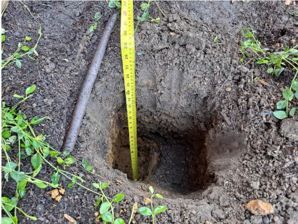
Plate 3: West side – thickness of clean cover. 0.50m topsoil underlain by 0.24m of subsoil with orange geotextile membrane
