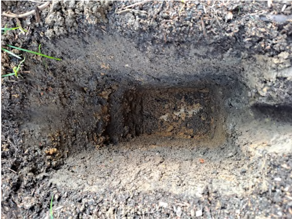
Plate 9: East side - trial hole. 0.41m of topsoil and 0.09m of subsoil (location on a podium over the basement car park)
