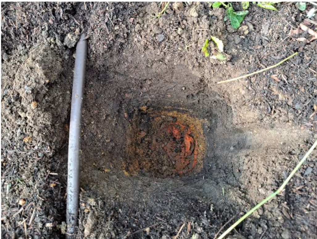
Plate 12: South side – trial hole. 0.35m topsoil underlain by 0.1m of subsoil with orange geotextile membrane
