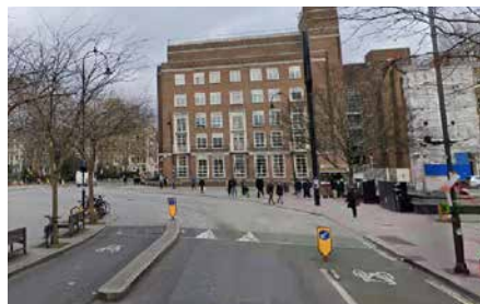
Transition from an active travel corridor to a flexible space at Byng Place, London. The consistent surfacing material and levels between the carriageway and footway give pedestrians priority and cue drivers and people on bikes to slow down.
