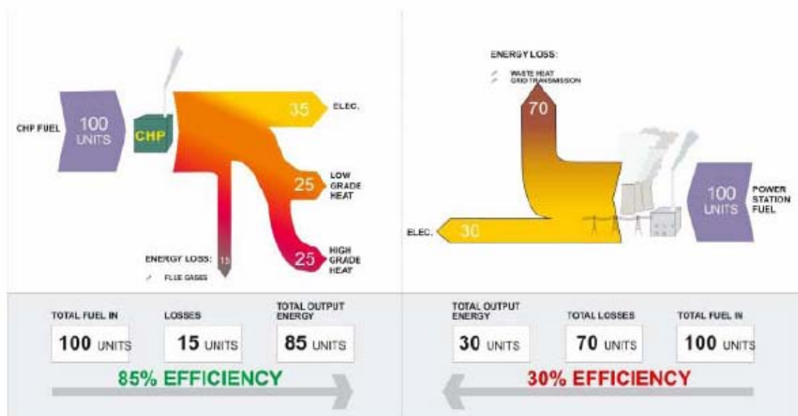
Figure 4.6 – CHP generation vs Conventional Power generation.
