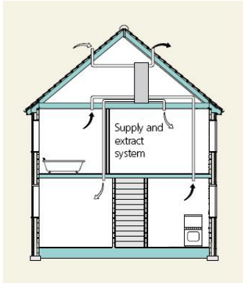
Figure 4.5. Whole Mechanical Ventilation with Heat Recovery (MVHR)
