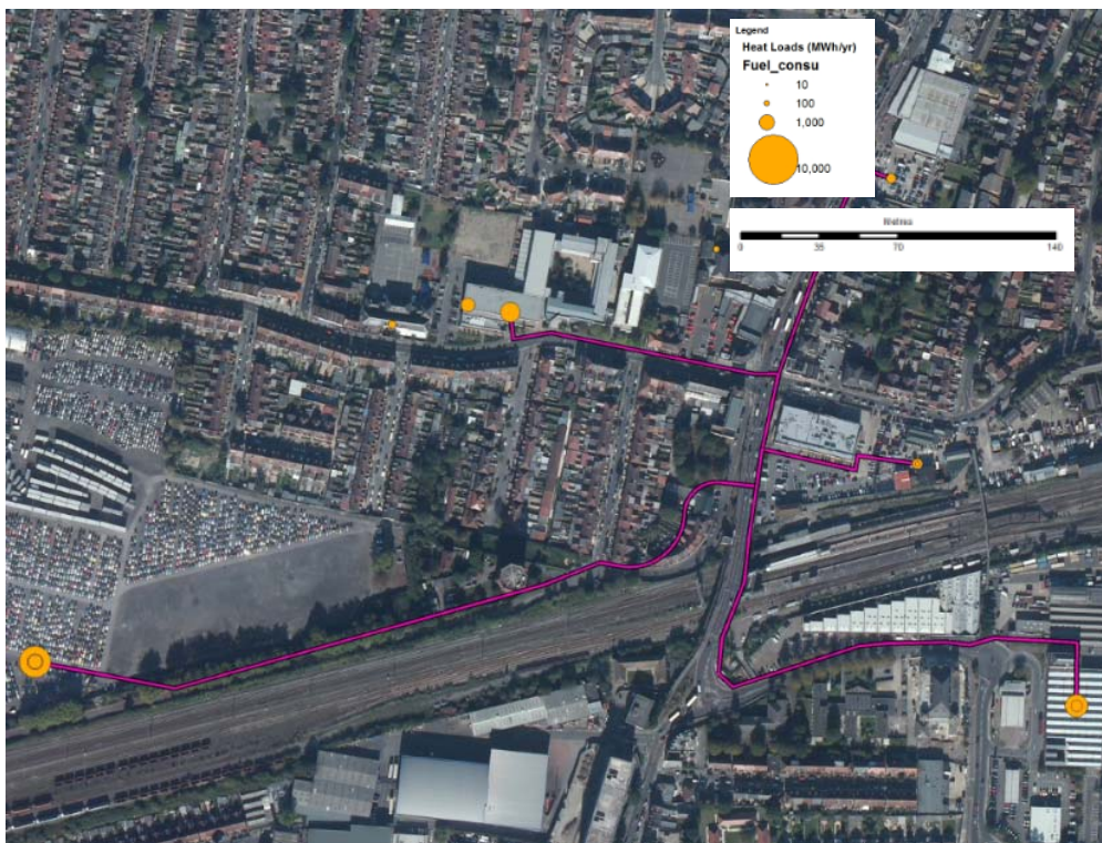
Figure A2.2: Core scheme refined based on route walk conclusions and load connection cost-benefit assessment
