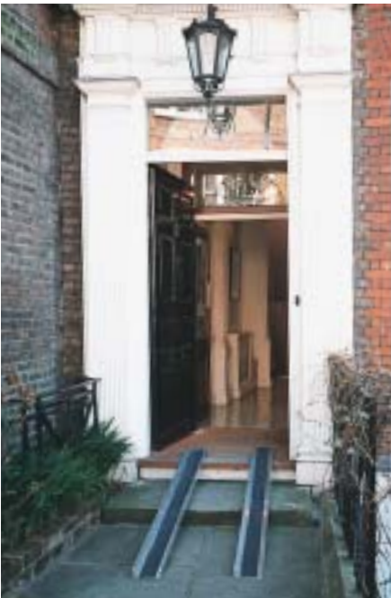
At St James' Church, Colchester, the level change at the north porch is more than a metre. The use of a removable ramp at the south door provides an adapted route during an interim period while a longer term solution is studied and funds raised to complete the alterations.
